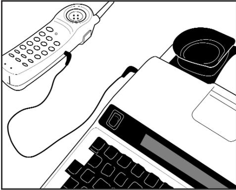
1. Connect the TDD to the cordless phone using the 2.5mm audible cable.
